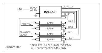
Note: When retrofitting with an instant start system to replace a rapid start system, some modifications to the socket wiring are necessary for optimal performance. This requires the two lamp pins to be shunted as close to the socket as possible. Do this by either installing shunted sockets or installing a jumper wire to tie the two lamp pins together in each socket. Failure to shunt the pins together will cause the lamps to fail prematurely.
